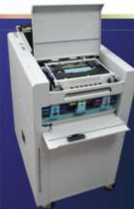
Easy access to Printhead and Ink Reservoirs
